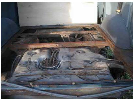
The rear floor is out, the back cross member is almost off, just tidying up the last bits. I will need to scrape down the chassis and other bits while the floor is out, ready to give it a coat of under seal.
