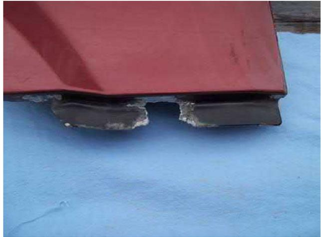
The front wings have the usual bit broken away at the bottom, where a bracket attaches them to the front bumper. A quick fix can be made by pop riveting a piece of aluminium to the wing, but it is a bodge and I would like to learn how to weld a new piece in. Perhaps David Ashburner has learnt how to weld aluminium during his Classic Car Restoration course at the Leeds City College?.
